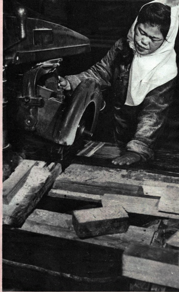
Toyo-ko Hanagusuku, 20, whose father was killed in the battle for Okinawa, runs this power saw making frames for prefabricated huts
